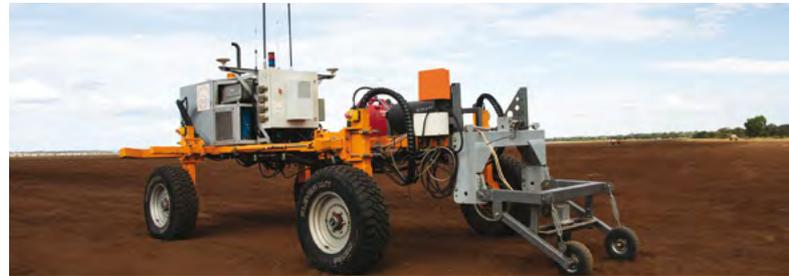
**Having several small microwave units teamed with the Weedit sensors and mounted on a robotic platform removes the time and power constraints that have so far prevented microwave weed control being a realistic option for broadacre operations.**
