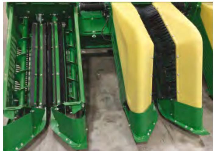
Photo 2: Stripper type harvester.
