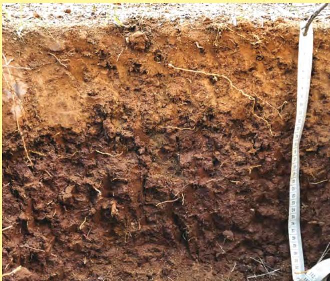
**FIGURE 2: The red rice soil exhibiting a massive, hardened structureless mass in the top 30 cm of the profile**
