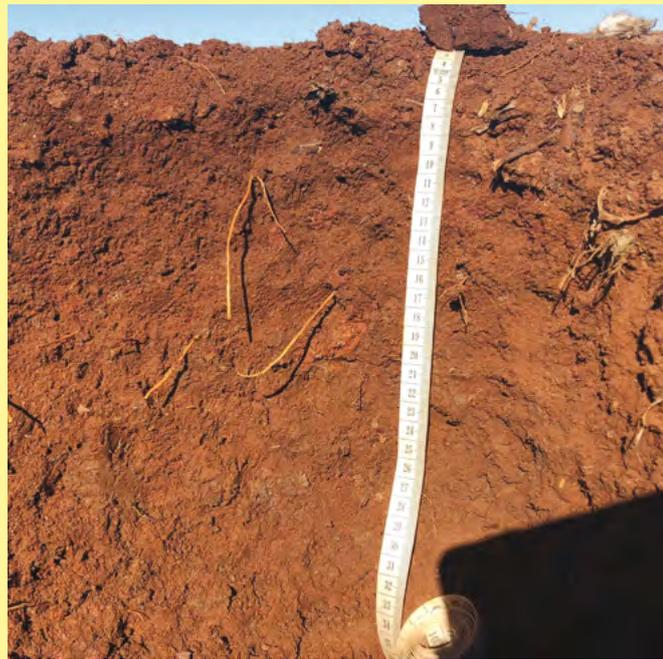
**FIGURE 4: An example of interconnected macropores and strongly pedal structure on the longer-term red cotton soil**
