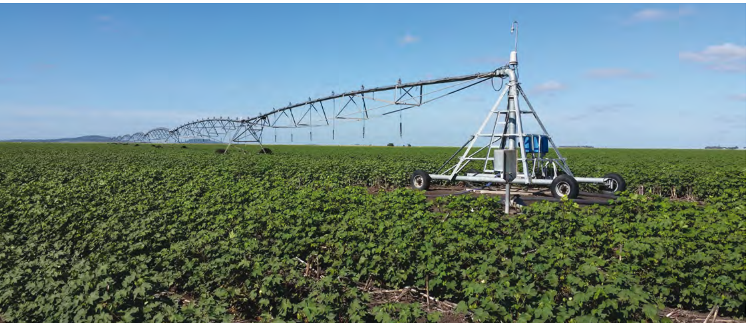
Variable-rate centre pivot irrigation machine on the Darling Downs.
