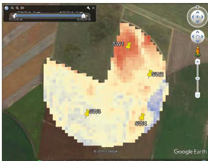
**Electrical conductivity map and location of soil moisture sensors on irrigated cotton crop.**
