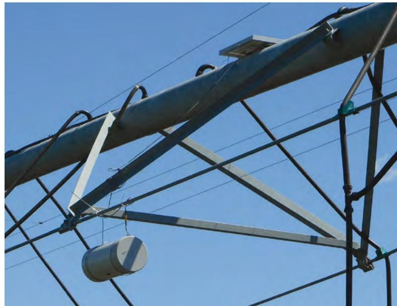
**Machine mounted crop camera collecting imagery of cotton cover and fruiting as machine passes over field**
