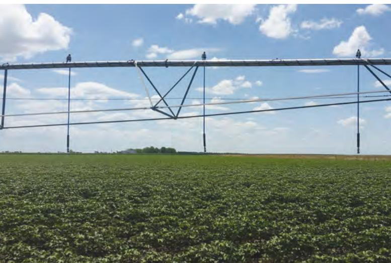
**Individual sprinkler variable-rate hardware on centre pivot irrigation machine.**
