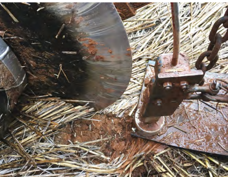
Photo 1: The South Australian NoTill Farmers Association conceived the AquaTill ‘Liquid Coultter’ as a means to slice cleanly through moist residue using aqueous liquid fertiliser. (SOURCE: Greg Butler 2016)
