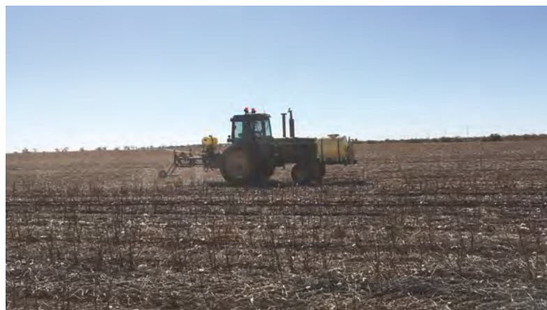
Photo 2: Testing the AquaTill ‘Injecticide’ on cotton ratoon using PTO driven FLOW Hyplex pump and the Injecticide engagement tool being developed by NDF. (SOURCE: Greg Butler 2018)
