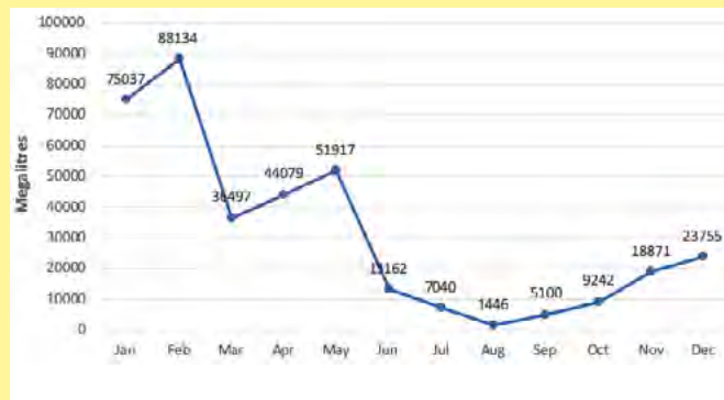
FIGURE 1: Mean amount of inflow for Nogoa River at Craigmore (28 years of data)
