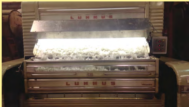
FIGURE 2: VIPR system installed on a gin stand at a commercial cotton gin during the 2018–19 ginning season in Meadow, Texas
