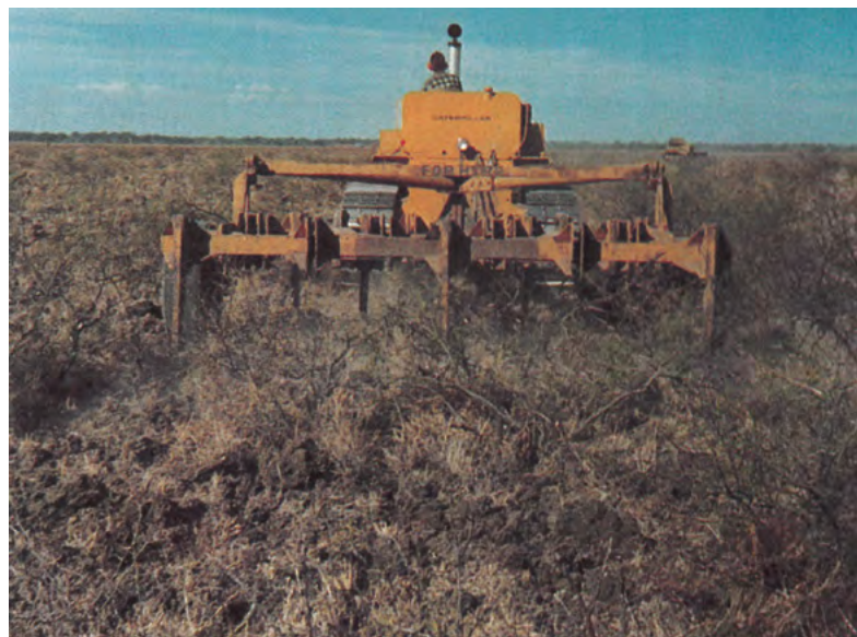
Auscott Midkin manager Don Davis gave advice on land preparation – "Deep rip to break up the surface."
