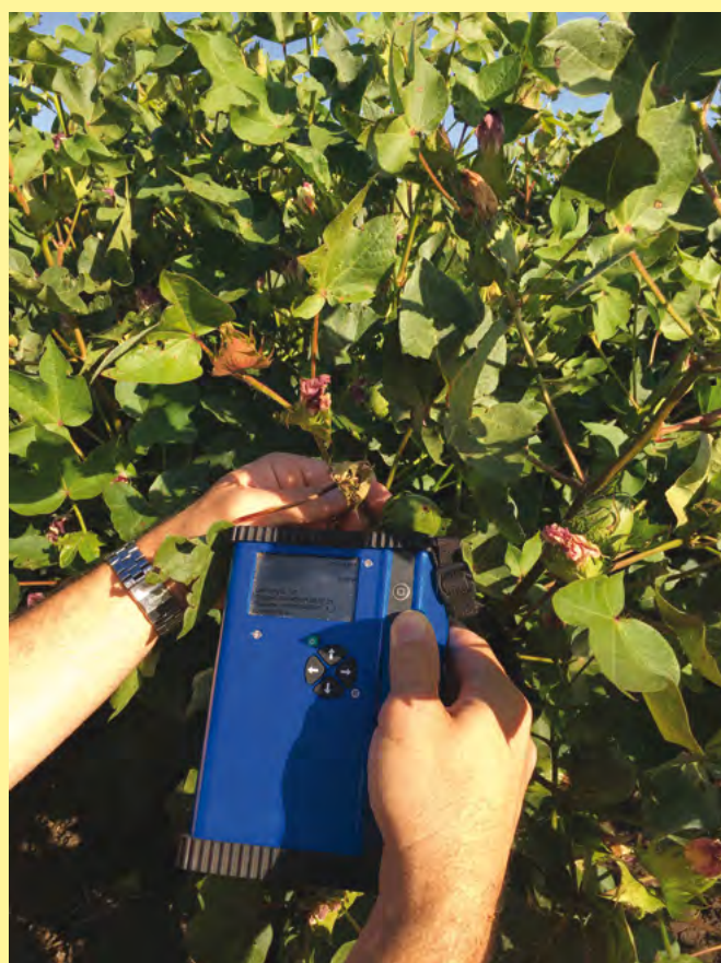
FIGURE 4: Using a Felix F-750 Produce Quality Meter to acquire NIR spectral information from a cotton boll in a commercial crop
